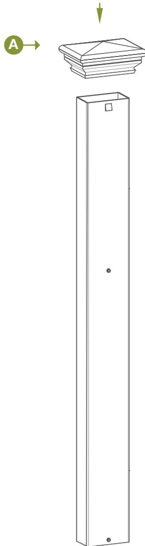
**Note:** The top of the post can be trimmed down as necessary. Use PVC glue (NOT INCLUDED) to permanently install the post cap as necessary.
