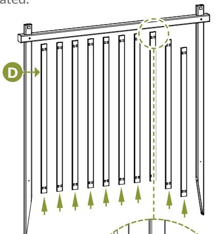
**Note:** Once inserted, the pickets will lock into place. To remove the pickets, gently insert a butter knife into the picket hole as shown and slowly pull up the picket(s).
